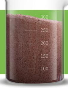
The FluMET is a cerium based regenerable adsorber that can be used to remove Fluoride contamination from drinking and industrial water (steel, aluminium, fertilizer, semiconductor, coal fired power plants, glass production, manufacture of fluorplastics, etc.).
