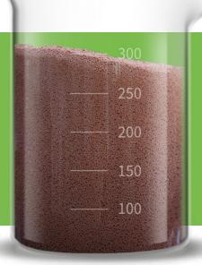
We offer a new, cost-effective, sustainable, and economic water treatment technology over conventional and chemical-intensive arsenic mitigation methods, it is called AsMET. AsMET is a cerium-based regenerable adsorber that can be used to remove arsenic contamination from drinking and industrial water. Regenerable means that as the adsorbent reaches its capacity limit, the media goes through a simple regeneration wash-off process and is ready to be used again for up to 10 years.
